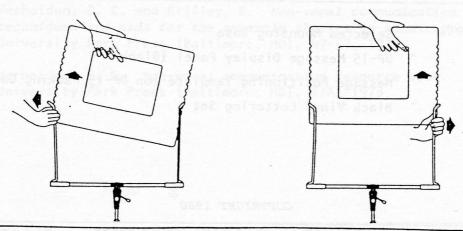
IMPORTANT: Pulling too hard on these rails (or long-term, repeated height adjustment of the panel) may bend the rails outward beyond their present spring ability. If this happens, remove the panel and exert just enough inward push to return the rails to their original position -- until they are again snug against the panel.
