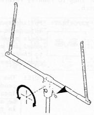
THUMB SCREW: (located mid-point on Swivel Assembly; beneath wing screw) \*
