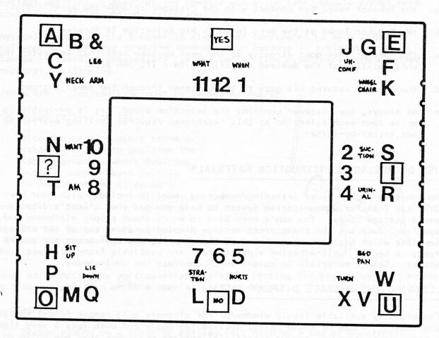
The placement of letters and numbers is very deliberate -- the most frequently used being put in units of easiest selection. Boxed items are primary use letters and, because of the highlighting, require only a one-gaze selection with eye return to the cut-out for confirmation.
